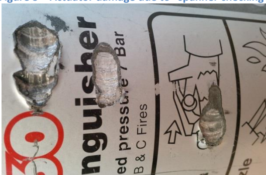
Figure 5 - Deep gouges in cylinder
